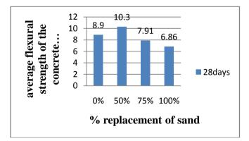
By this table and graphs shows that there is an increase in compressive strength, split tensile strength, flexural strength with 0%, 50%, 75%, 100% replacement of sand with quarry rock dust and it decreases with after 50% replacement in both M30 and M40 grade of concrete.
